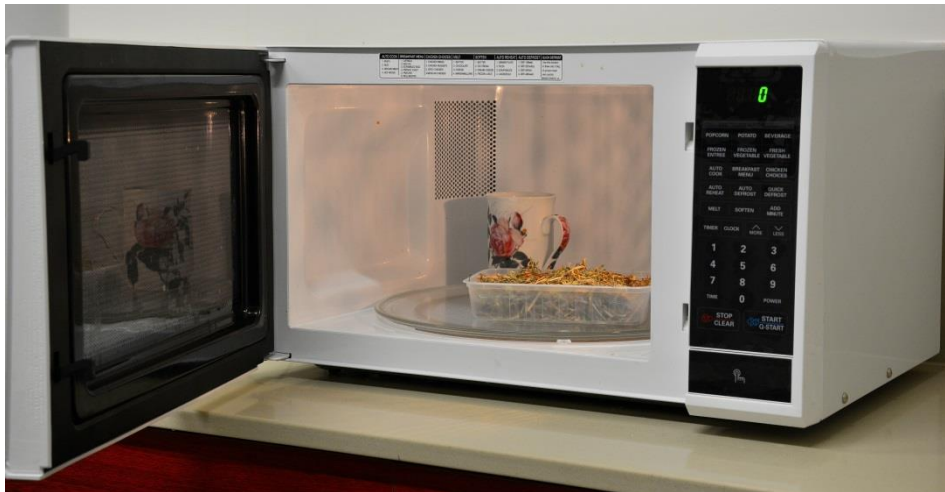
Estimating moisture in a hay sample using the microwave method
