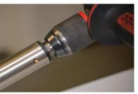
This piece attaches to a drill. DO NOT BELT THE END OF THIS WITH A HAMMER. THEY ARE HARDENED STEEL AND COME FROM BALLARAT AND WILL COST YOU A LOT OF MONEY TO REPLACE IF YOU DAMAGE IT.
